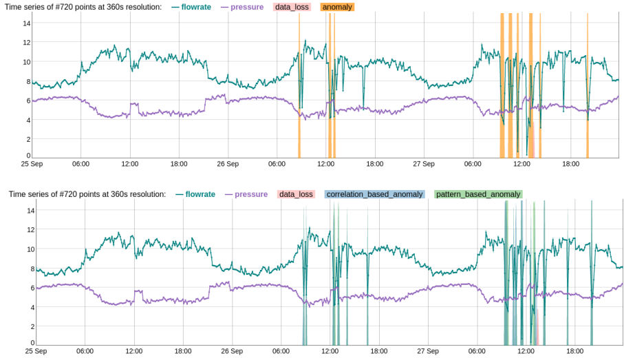
Figure 6.15: Example nontrivial anomaly #2. Combined (top), and with breakdown (bottom). Pressure rescaled for readability
