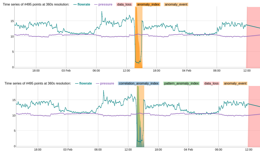
Figure 6.13: Example trivial anomaly #3. Combined (top), and with breakdown (bottom). Pressure rescaled for readability
